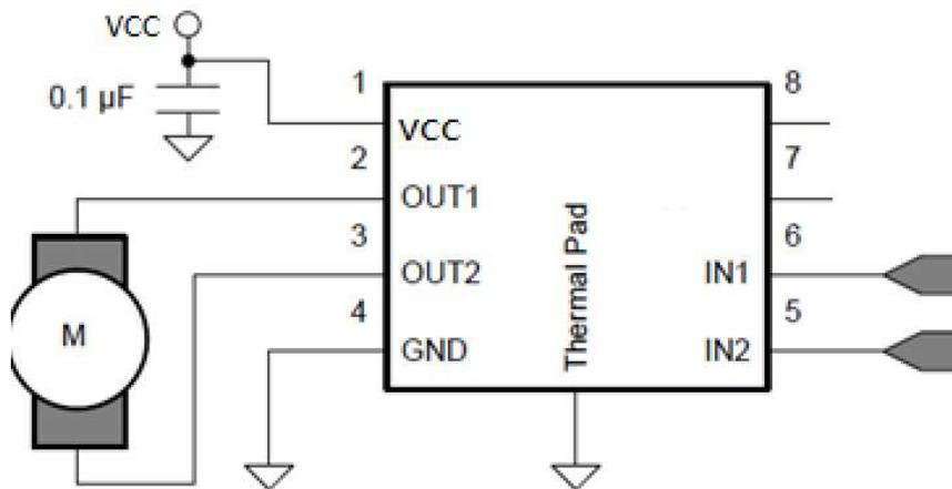
Figure 2. Schematic of SC8901 Application
