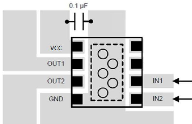
Figure 4. Simplified Layout Example
